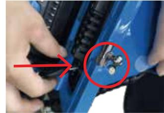
Unlocked-locking pin not protruding through frame
